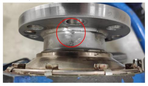
Fig. 7. Possible damage to the propeller shaft, when using tooling improperly.
